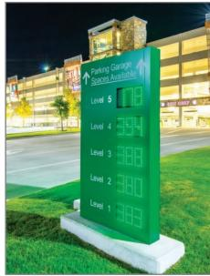
Walker Parking Consultants Wired and wireless sensors can monitor use of individual parking spaces throughout the facility to determine where open parking is available. That information is then wirelessly communicated and displayed via LEĎ signage at key locations.
