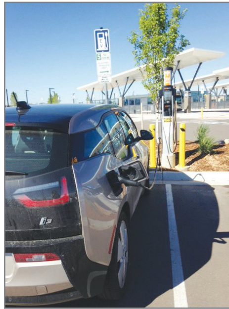
Kathy Pitts Standard Level 2 charging stations deliver 240 volts of electricity to a battery and provide vehicles with 10 to 20 miles per hour of charge, which is the appropriate level for multifamily housing, office parks and other places where cars typically are parked for two to six hours at a time.
