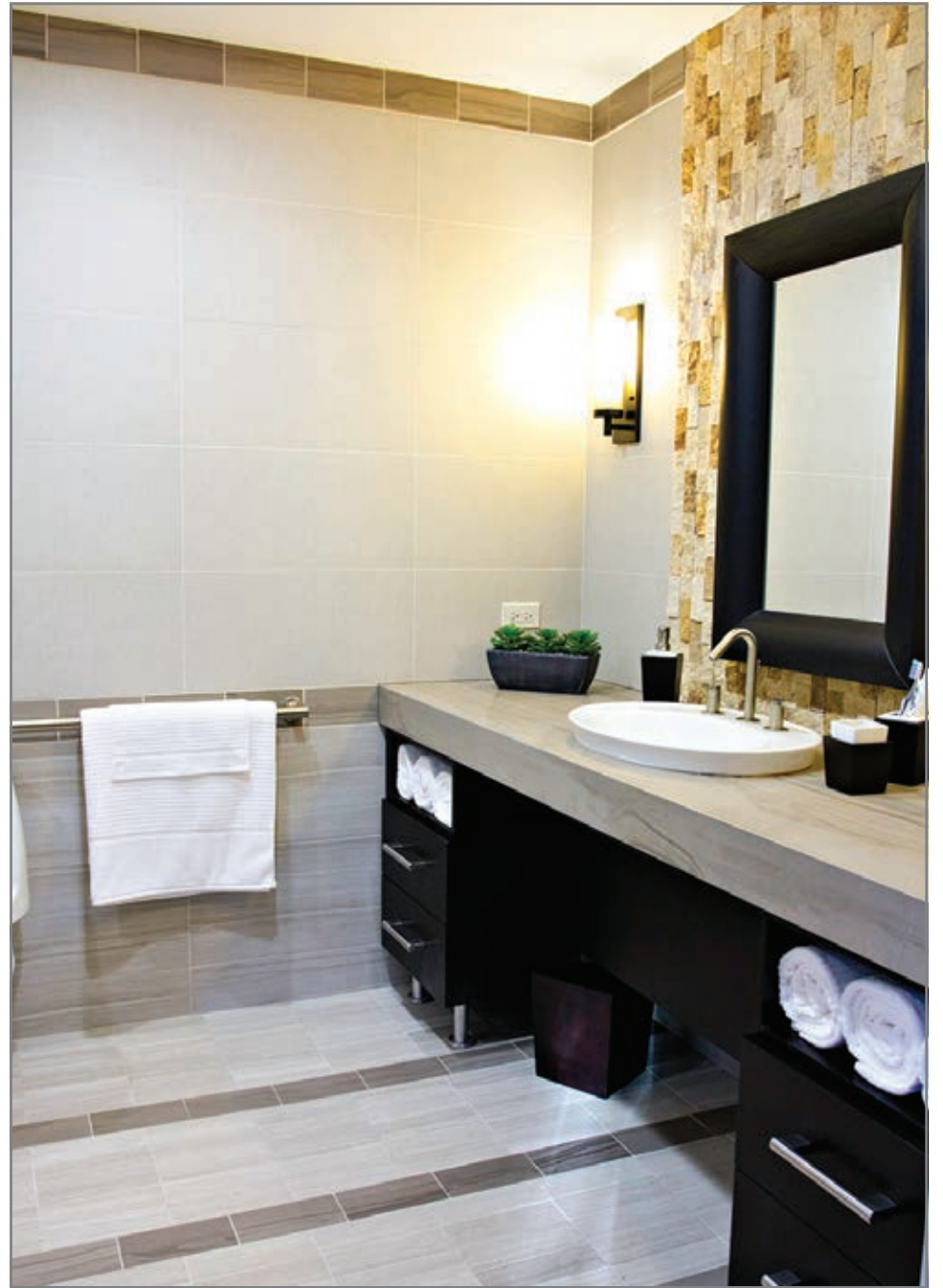
Grab bars look like towel bars, and the bath was designed to accommodate each phase of recovery – wheelchair to walker to walking.
